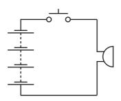
complete series circuit; battery of 4 cells connected correctly;
